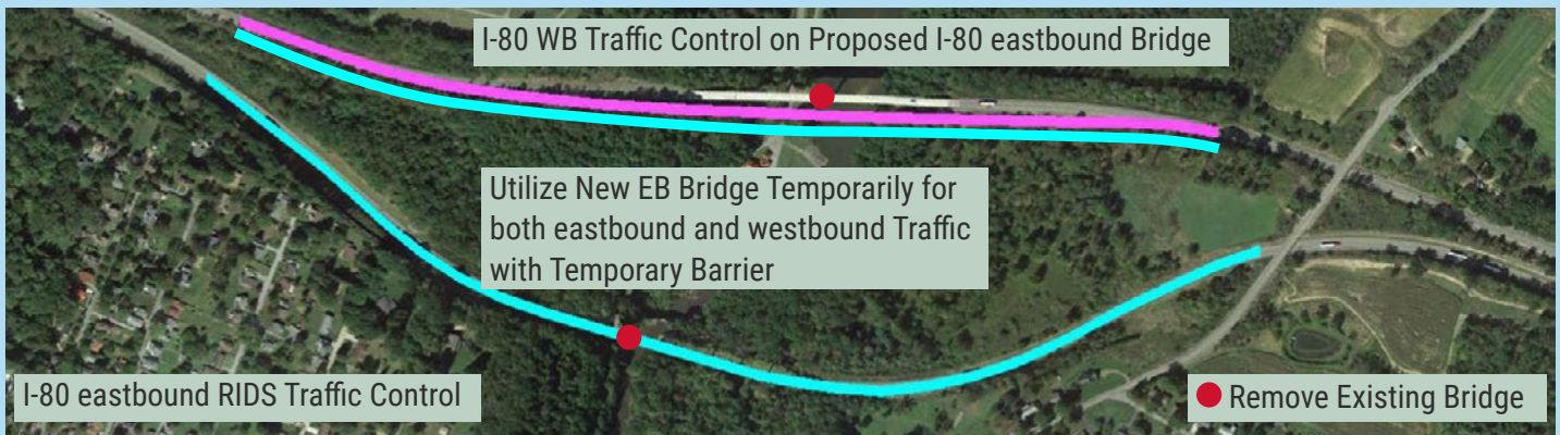
FIGURE 16 - ALTERNATIVE TRAFFIC CONTROL WITH CONCURRENT EXISTING BRIDGE REMOVAL AT I-80 NORTH FORK BRIDGES
